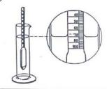
With the eye at the level of the surface of the liquid, the correct reading is 70, and NOT 66.
